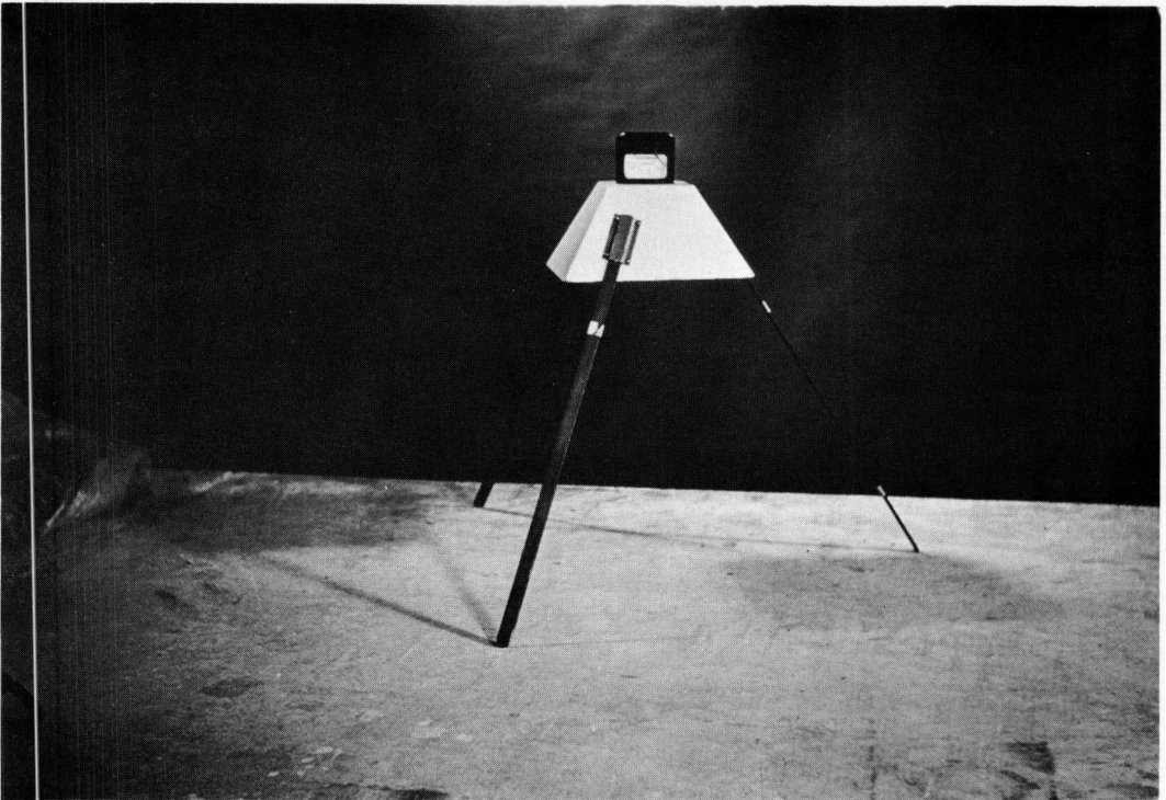
Figure 3. Apparatus for measuring light reflectance.
