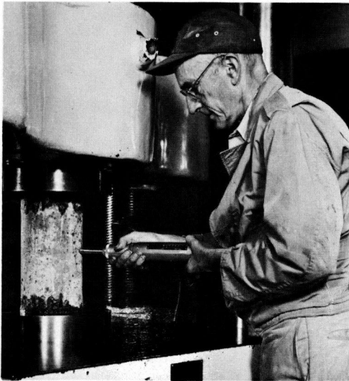
Figure 5. The Swiss hammer as used in the laboratory in series 2.
