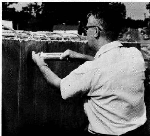
Figure 9. Swiss hammer being used in the field.
