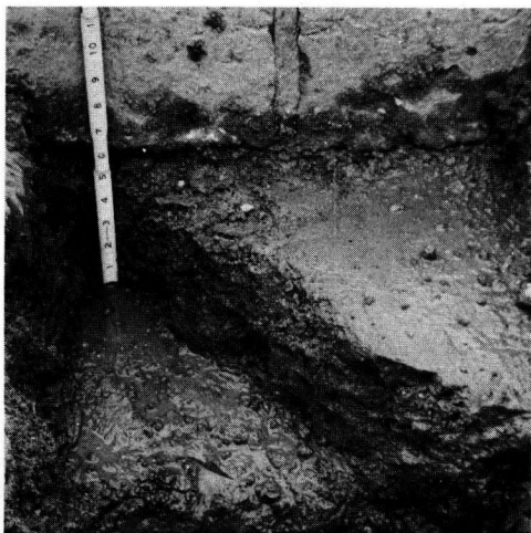
11 percent cement-modified soil at 1159 + 20
