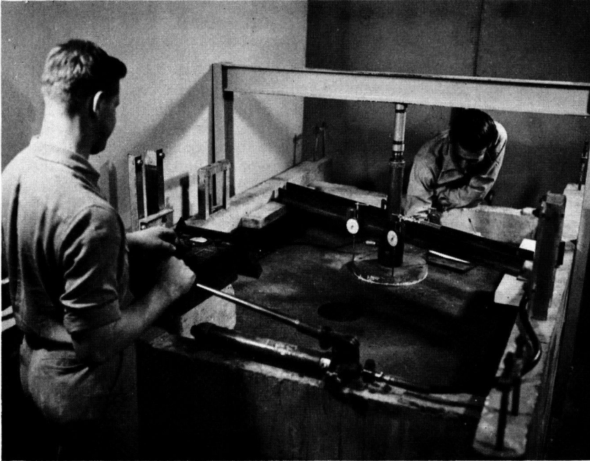
Figure 3. View of soil container with clay subgrade, subbase drains, and soil pressure cell in place. A plate bearing test is being performed on the subgrade.
