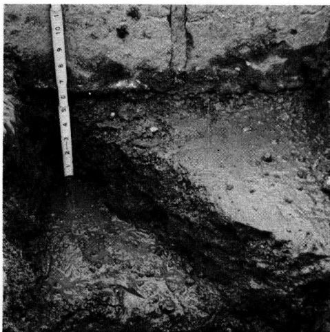
11 percent cement-modified soil at 1159 + 20
