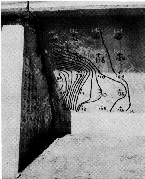
Figure 5. Relative deterioration measured by pulse velocity.
