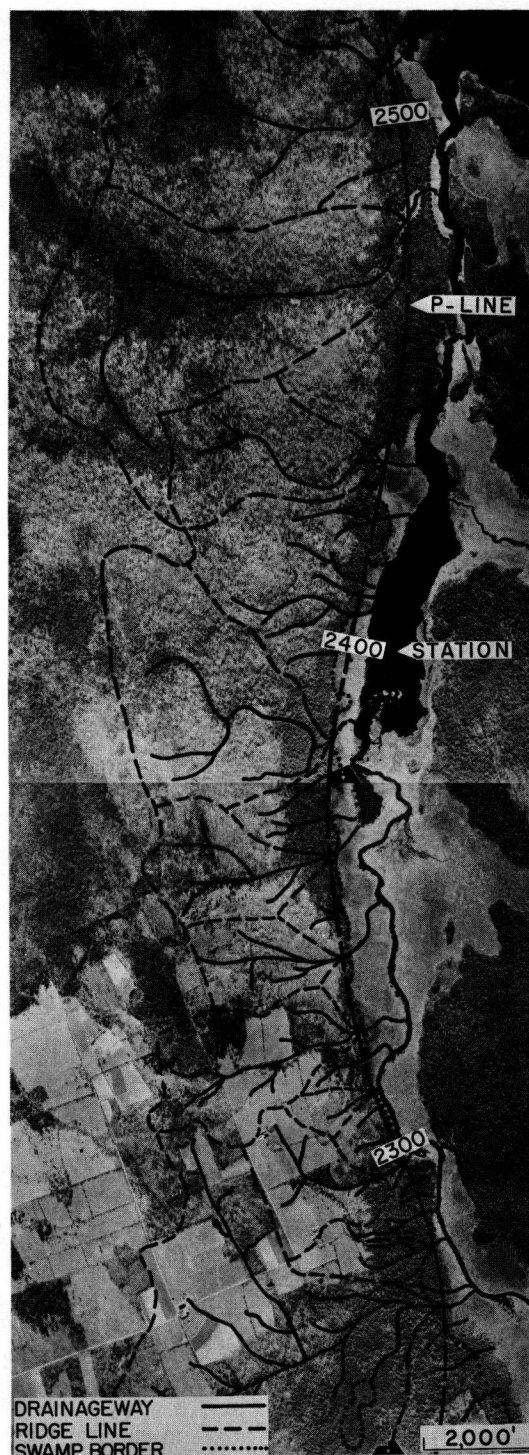
Figure 4. Uncontrolled mosaic of drainage delineations. Watershed areas were obtained directly from the photos.
