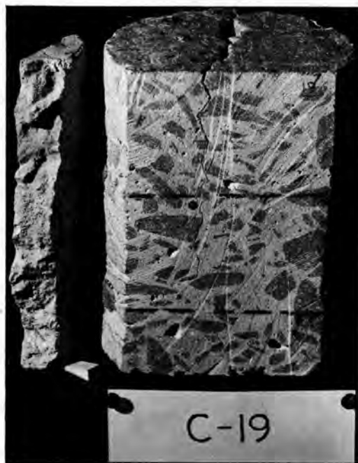
Figure 17. Core at crack in 8-in. section, Sta. 823+08.
