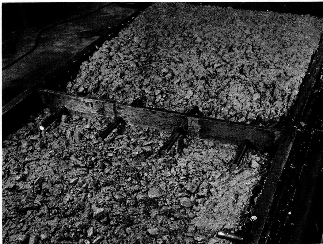
Figure 3. Appearance of concrete during fabrication of a specimen; fluidity was obtained with internal vibrators.
