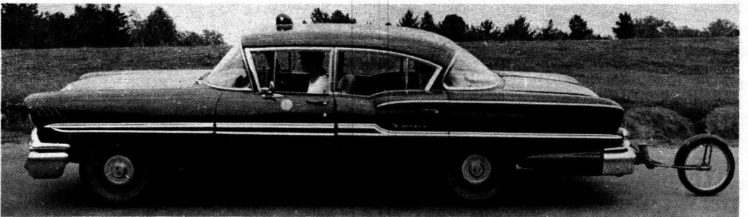
Figure 8. The skid test car used by the Virginia Council of Highway Investigation and Research utilizes no special braking equipment. Only recording equipment has been added to the commercial vehicle.
