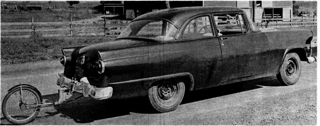
Figure 6. The car used by the Purdue Joint Highway Research Project eliminates irregular foot braking by utilizing a special vacuum braking system activated by a hand microswitch (4).
