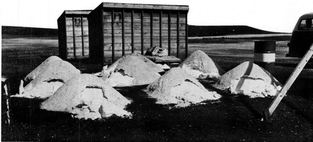
Figure 5. General view of Field Test B, with various mixture stockpiles that had been tarpaulin covered and observed for two months. Storage tests were also conducted in sheds at rear.
