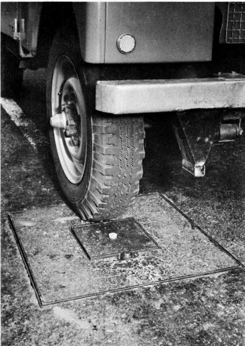
Figure 2. Close-up showing stress-recorder in position.
