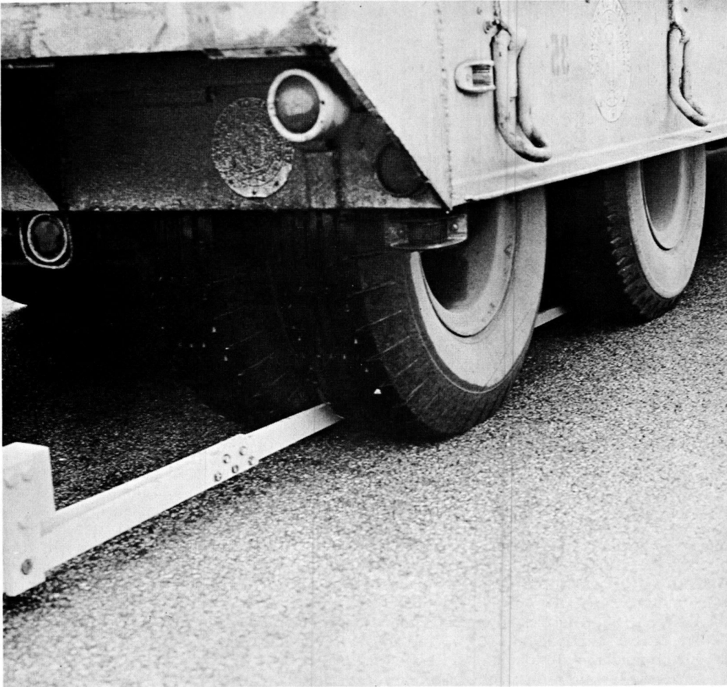
Figure 14. Benkelman Beam in-place for measuring pavement deflection under 32,000- or 36,000-lb loads on tandem axles.
