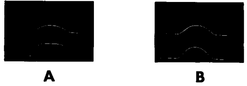
Figure 8. Typical force recordings showing transverse and vertical traces. Chevrolet Brookwood (loaded): rear wheel; tire, 8.00-14; wheel load, 650 kg; stud height, zero; inflation pressure, 2.8 kg per sq cm.
