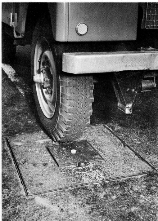
Figure 2. Close-up showing stress-recorder in position.
