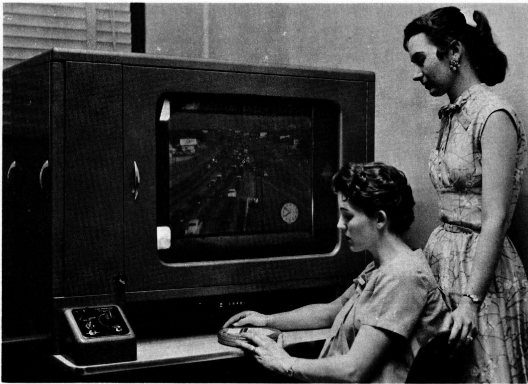
Figure 3. Time-motion study projector used in analysis of motion pictures.
