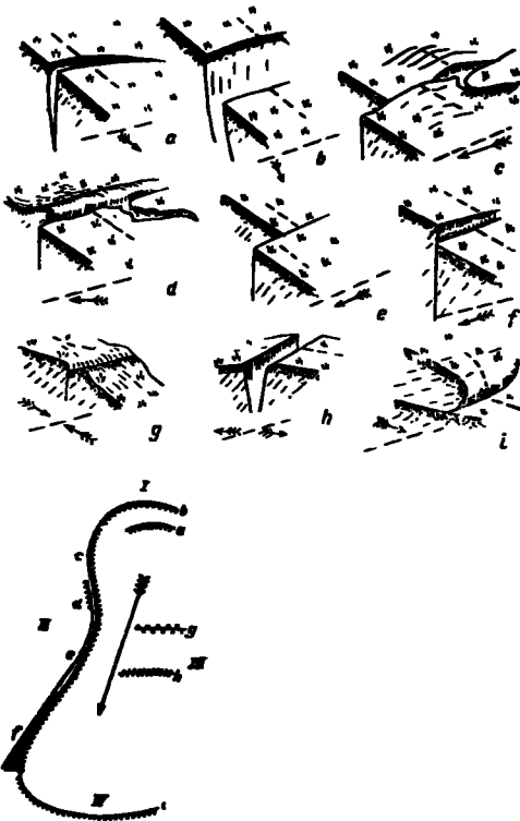
Figure 1. Types of cracks on a slide.
