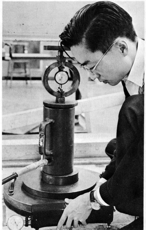
Figure 6. Measurements of surface strains and crack widths.
