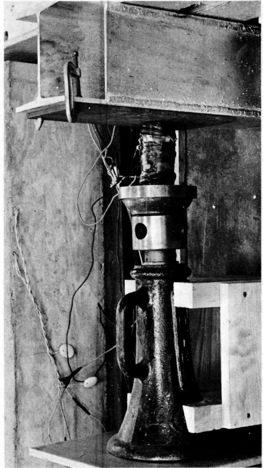
Figure 8. Longitudinal load jack and cell.
