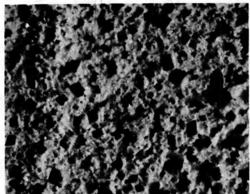
Figure 21. A close-up (x60 magnification) showing perfect "casts" of dolomite rhombs which were etched from the silicified shell zone. Compare with Fig. 19.
