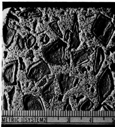
Figure 14. An acid-etched section taken from the same test bar as the section shown in Fig. 11, after only 30 days (as opposed to 60) in environment B.
