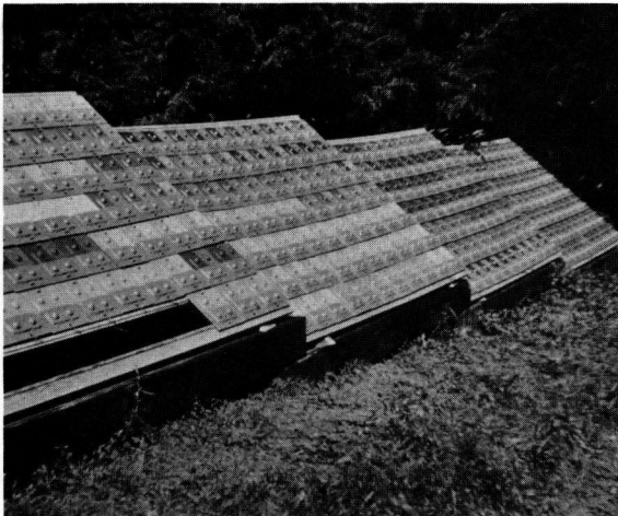
Figure 9. Testing additives to synthetic resin paints—designed to combine wetting with durability. Fabricated panels have rivets, crevices and welds.
