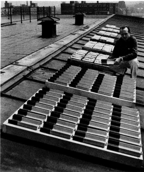
Figure 8. Exposure of 16 paints in which rust was substituted for commercial iron oxide.
