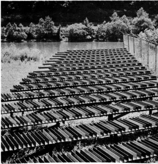
Figure 6. Test panels for determining best methods for painting of welds. (Neville Island, Pittsburgh, Pennsylvania.)
