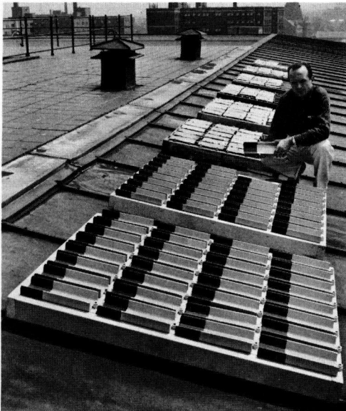
Figure 8. Exposure of 16 paints in which rust was substituted for commercial iron oxide.
