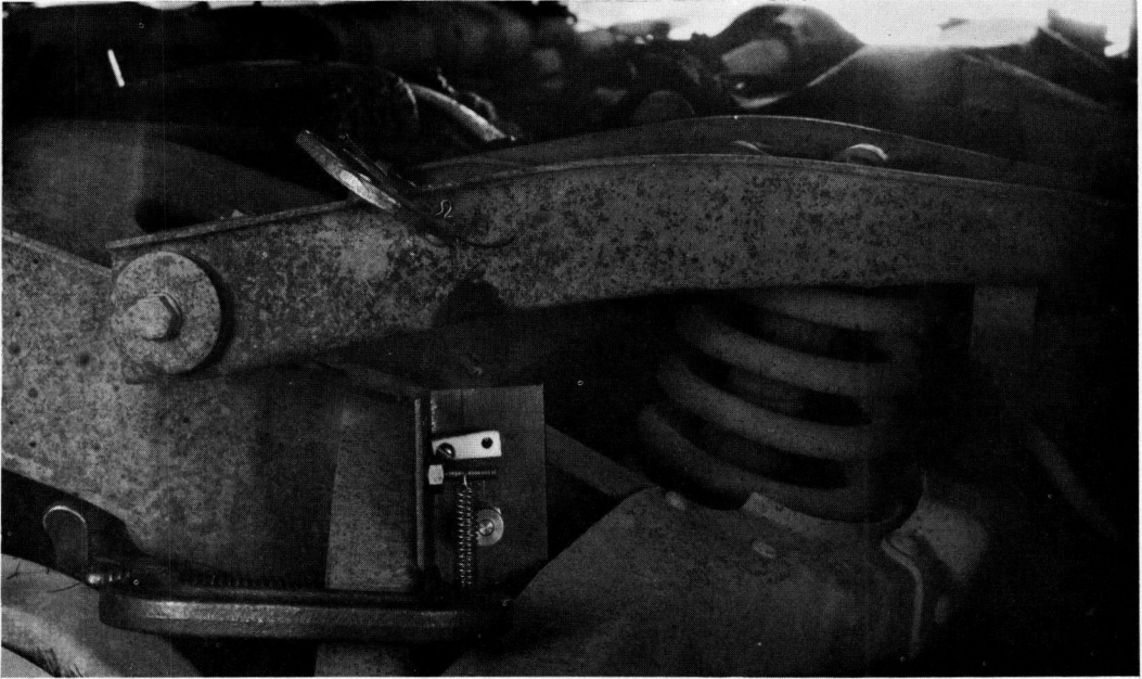
Figure 9. Transducer mounted on vehicle.
