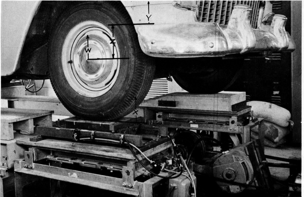
Figure 4. Front wheel of vehicle mounted on vibrator.
