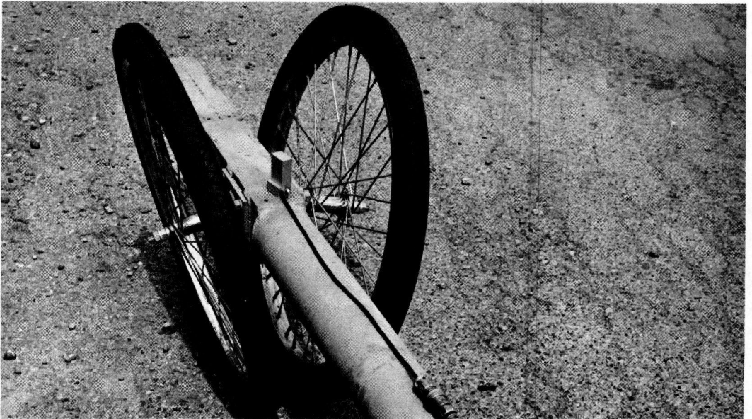
Figure 2. Accelerometer mounted on trailer.
