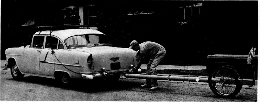
Figure 1. Trailer for making highway profile measurements.
