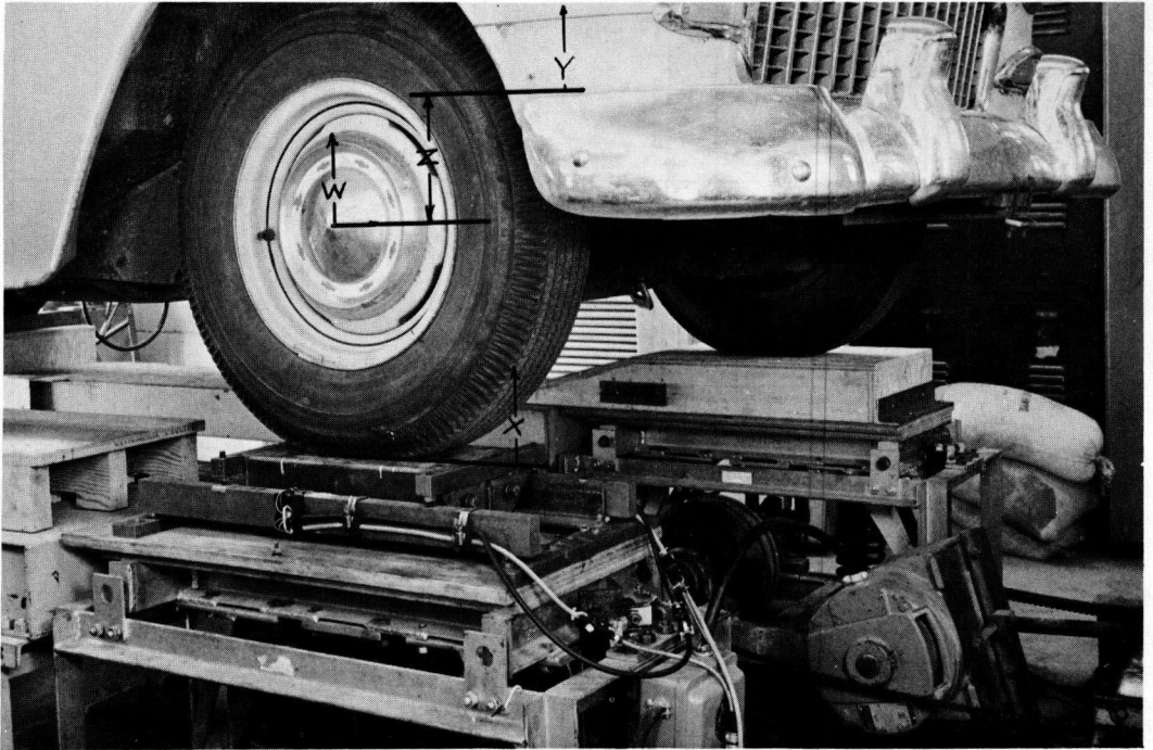
Figure 4. Front wheel of vehicle mounted on vibrator.
