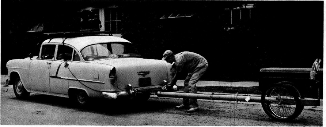
Figure 1. Trailer for making highway profile measurements.
