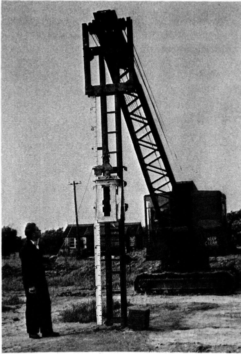
Figure 5. General view of the equipment used in the investigation of impact compaction. The rammer has been raised to a height of about 5 ft and the operator is about to trip the quick-release mechanism.
