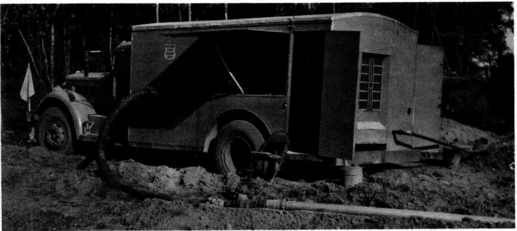
Figure 7. Truck-mounted 1,000-gpm pump.
