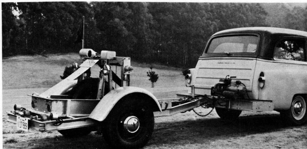
Figure 7. BPR Road Roughness Indicator, outrigger trailer carrier and tow car.
