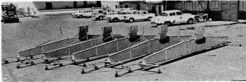
Figure 47. Most recent California model—hand-propelled recording Profilograph intended primarily for construction control.
