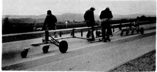
Figure 44. Hand-propelled Profilograph with unitized frame for rapid knockdown.
