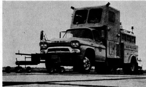
Figure 30. Michigan Profilograph unit modeled after the California Design shown in Figure 41.
