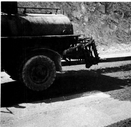
Figure 14. Curing seal "boot truck".
