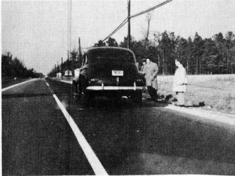
Figure 8. Skid Tests on Sand Asphalt Surface - Note mark on pavement and dust from chalk bullet fired by detector as wheels were locked.
