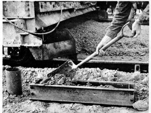
Figure 28. Taking beam samples for modulus of rupture tests.
