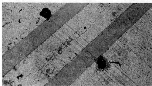
Figure 45. Plugs set in epoxy resin for crack opening measurements.
