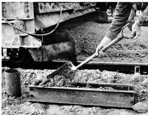
Figure 28. Taking beam samples for modulus of rupture tests.
