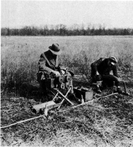
Figure 2. Apparatus Used by the Bureau of Public Roads in Shallow Earth-Resistivity Operations
