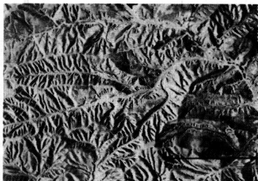
Figure 32. Drainage Pattern of Loess - Left - Airphoto of Area in Lincoln County, Nebraska - Right - Drainage Map of Same Area
