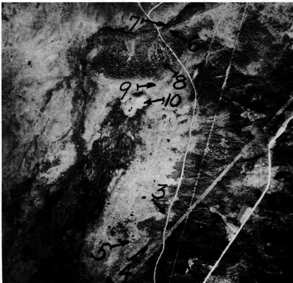
Figure 21. This vertical airphoto contains some of the major topographic features contained in the diagrammatic sketch of Figure 20. It covers the upper portion of valley fill to the outward part of the valley fill. The arrows point out the following features associated with the lower topographic portions where permafrost conditions vary:
