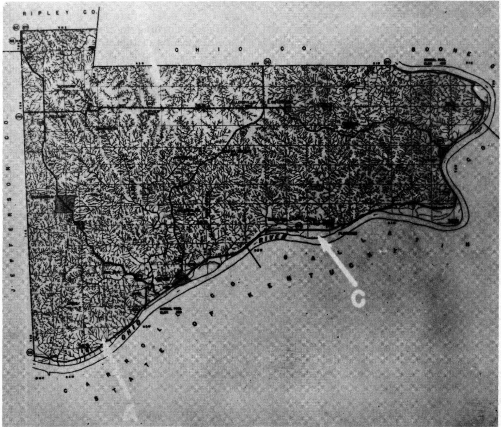
Figure 35. The drainage map of Switzerland County, Indiana, exhibits the following drainage patterns: "A" - Dendritic drainage pattern of Ordovician limestone-shale regions (See Fig. 2 and 7). "B" - Subdendritic drainage pattern of Illinoian glacial drift regions (See Fig. 3 and 18). "C" - Weakly developed dendritic drainage pattern of river valley granular terraces (See Fig. 22). (This map was compiled from aerial photographs in the laboratories of the Joint Highway Research Project at Purdue University, Lafayette, Indiana. Scale: Typical square of grid system equals one sq. mi.)
