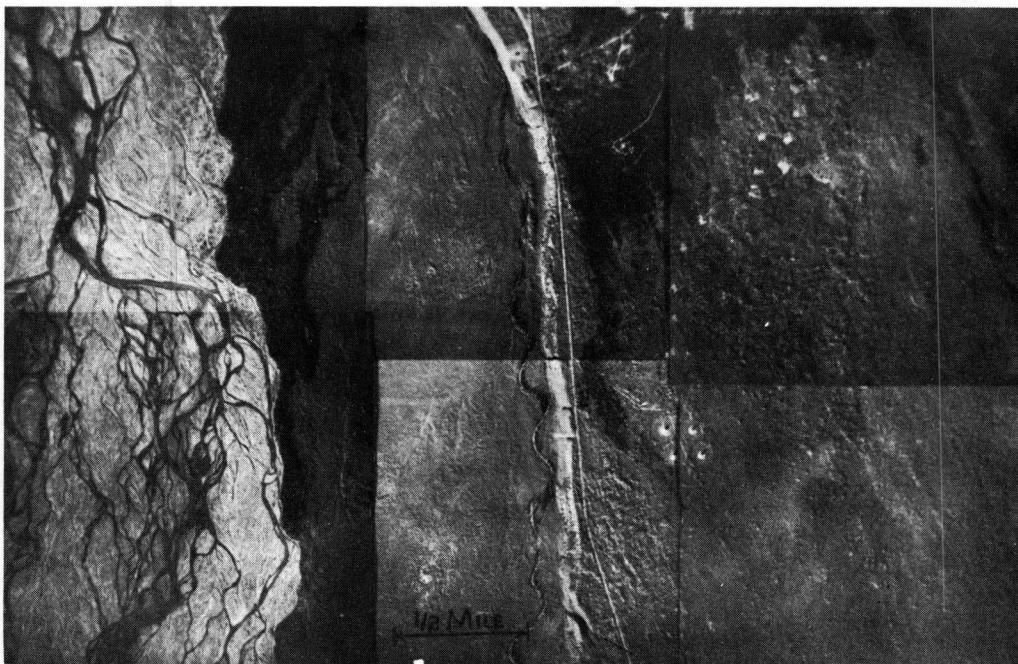
Figure 28. This airphoto contains many of the identifying elements of a good engineering location - that of frost-free granular materials.
