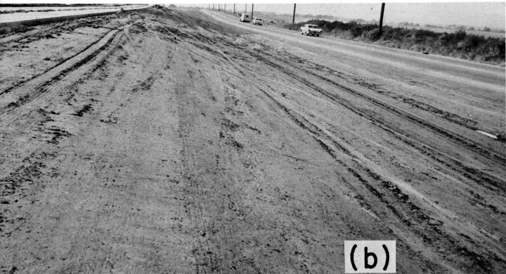
Figure 6. Appearance of test sections, 24 hours after application: (a) asphalt mixing solution—1:10 section in foreground, petroleum resin 1:7 section in background; (b) untreated section in foreground, lignin sulfonate 1:10 section in background.
