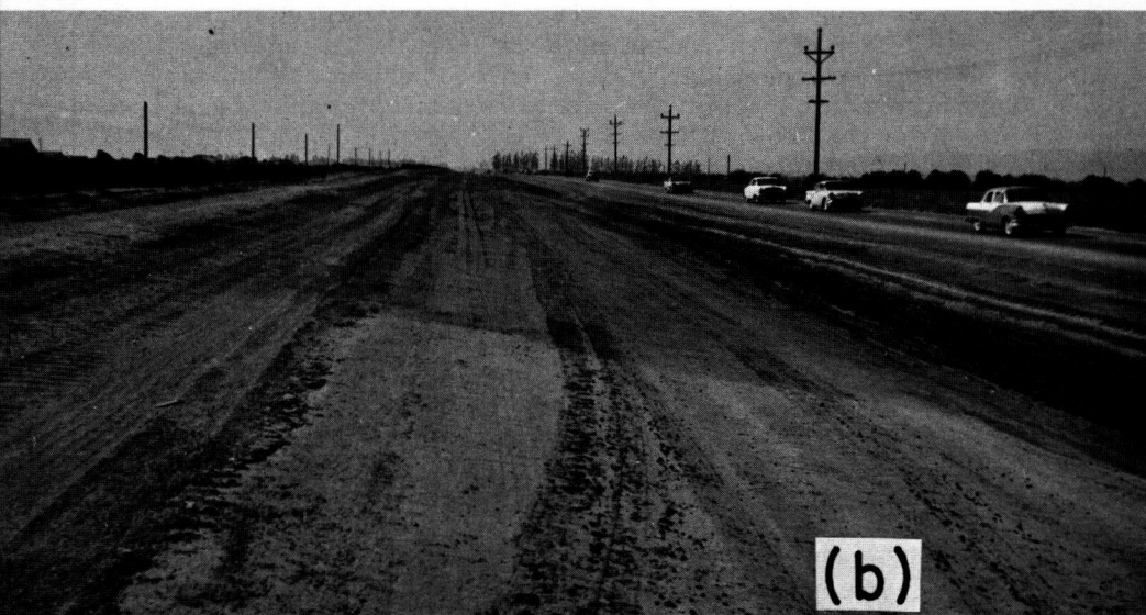
Figure 7. Lack of dust formation over treated sections: (a) asphalt mixing emulsion 1:30—shows an area where the most severe dust formation was encountered on the job; (b) asphalt mixing emulsion, 1:10 background, petroleum resin 1:7 foreground. These photographs were taken approximately 48 hours after treatment with a wind velocity of 20-25 mph. Compare with photograph shown in Figure 5.
