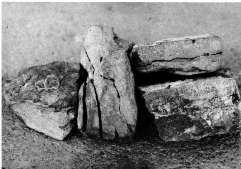
Figure 10. Clinkers following exposure to accelerated weathering test. The two pieces on the left were exposed for 28 days of alternating heat-spray-rest cycles. The samples on the right were subjected to spray-freeze-rest-heat cycles.
