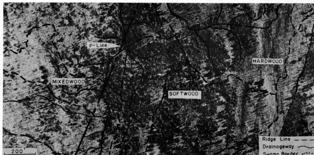
Figure 3. Drainageways and ridge lines visible beneath different forest types on an airphoto taken in early spring before foliage on deciduous trees was developed.
