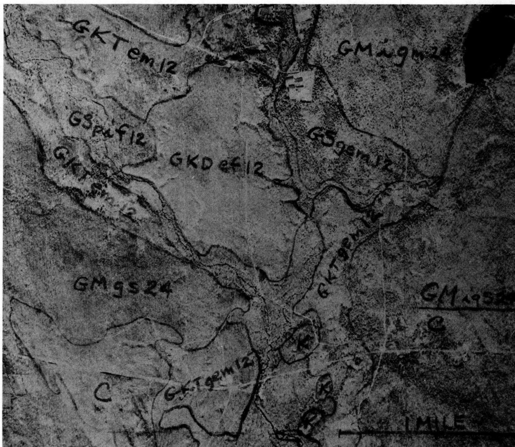
Figure 1. The soil borders were marked on the airphotos with a red wax crayon. The area marked "C"—crystalline rock—is an area with so much rock outcropping that it is essentially a non-soil area.
