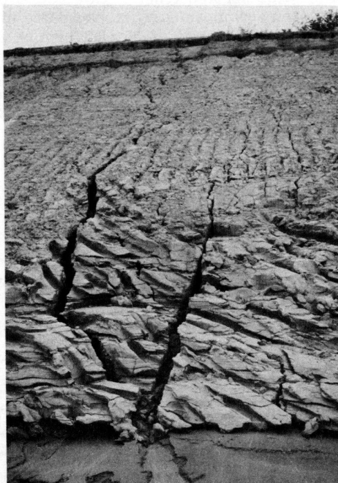
Figure 13. Tension cracks at toe of slope, resulting from bulging.
