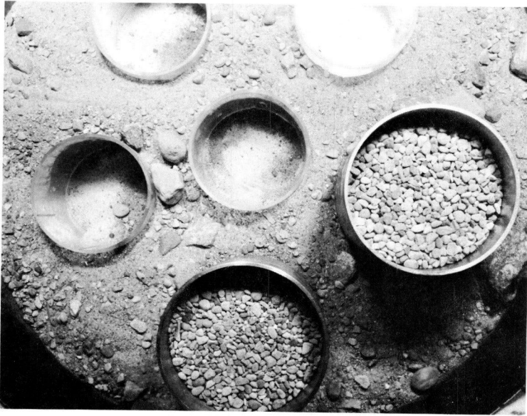
Figure 8. Container holding 6 samples, 2 in brass and 4 in lucite cylinders.
