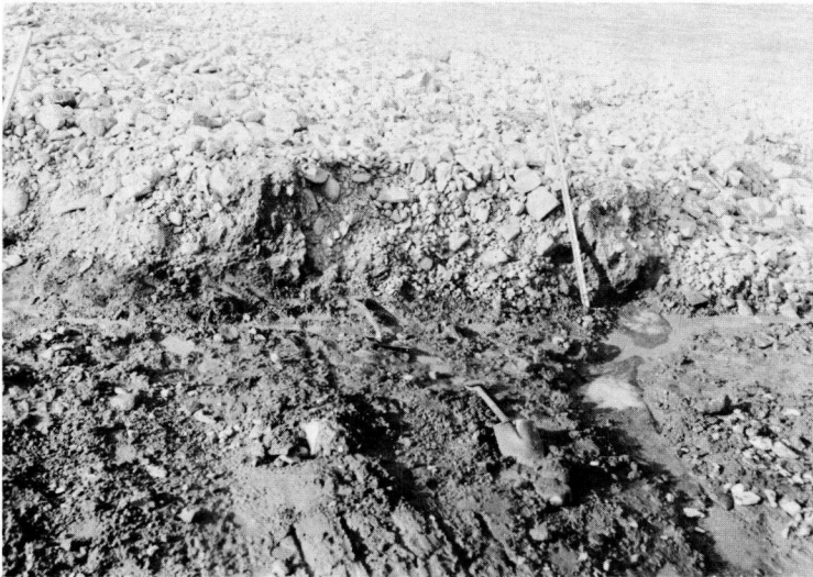
Figure 26. Vertical sorting on slopes, Thule area. Scale rests on ice wedge in permafrost. Coarse particles below shovel, cave in trench.
