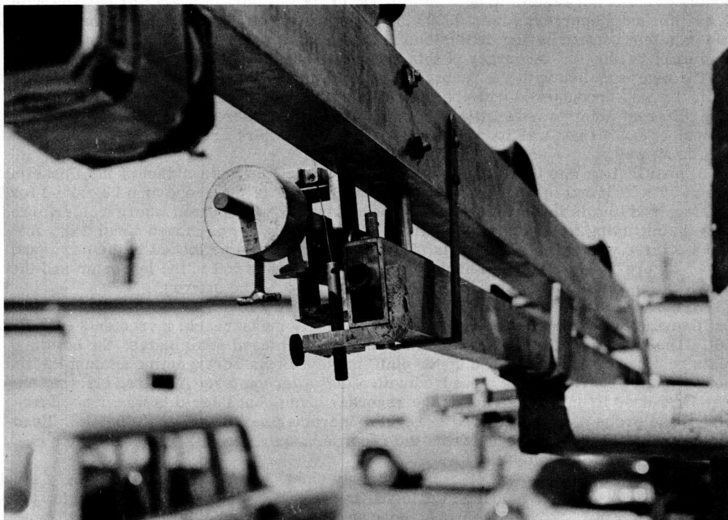
Figure 13. Satisfactory recorder arm linkage.
