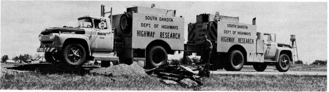
Figure 4. Plate load test trucks.
