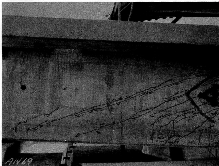
Figure 19. Cracking pattern, composite shear test, pretensioned beam.
