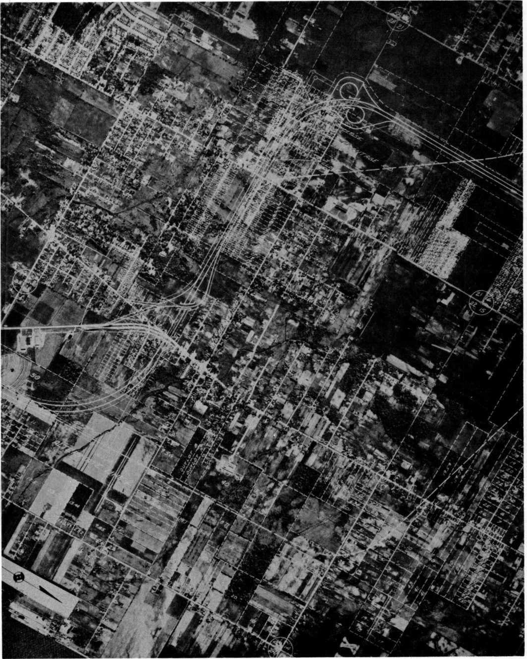
Figure 1. Portion of photographic mosaic used in location studies for Interstate 75 northwest of Detroit.
