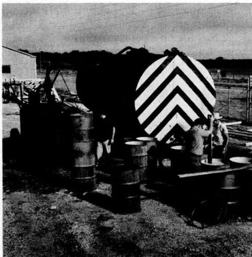
Figure 15. Recirculating asphalt heater and 10,000-gal storage tank used to mix Aliquat H226 solution. Aliquat H226 shipped in barrels shown in foreground.
