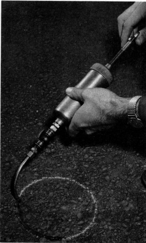
Figure 1. Performing permeability test: (a) forming grease ring; and (b) applying water solution to pavement surface.
