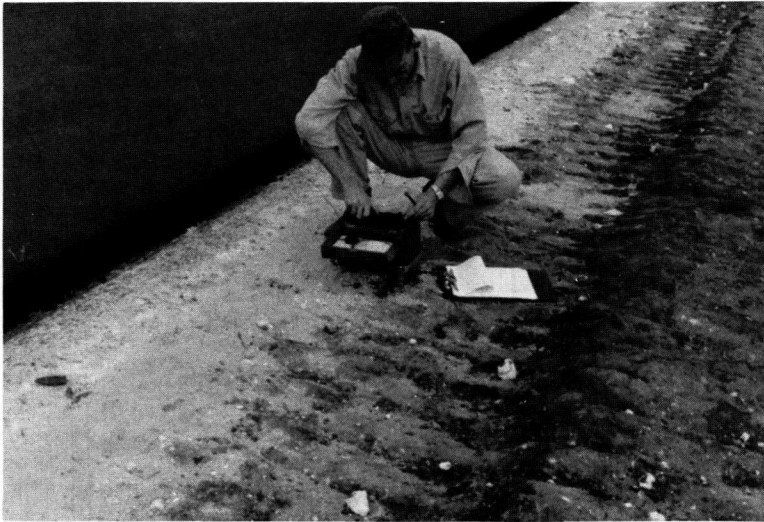
Figure 4. Thermocouple reading via a potentiometer calibrated to temperature in degrees fahrenheit directly.
