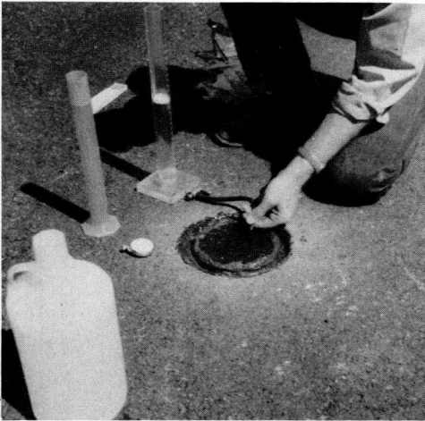
Figure V. Applying test solution to open graded surface within 6 in. diameter test area.
