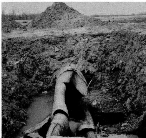
Figure 24. Failure of 96-in. 8 ga. corrugated metal pipe.
