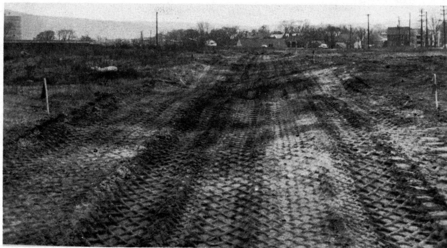
Figure 3. Test Strip 2 Following Rolling with 31-Ton Roller Showing Surface Irregularities Developed
