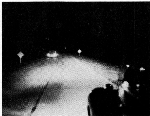
Figure 7. Photograph of Vehicular Encounter Using Polarized Headlights and Viewers.
