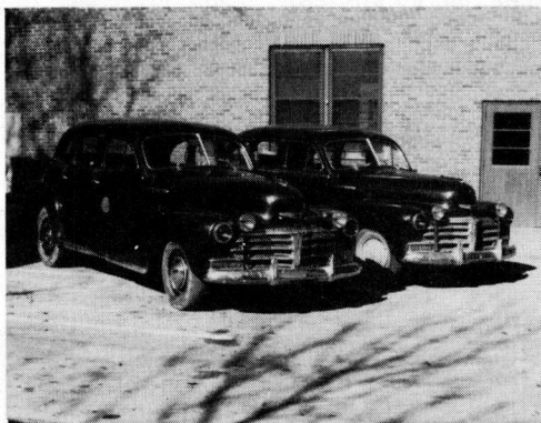
Figure 5. Two of the Cars Used in the Field-Testing Program. Both were equipped with polarized headlights, PAR-46 traffic lights, and polarizing viewers.
