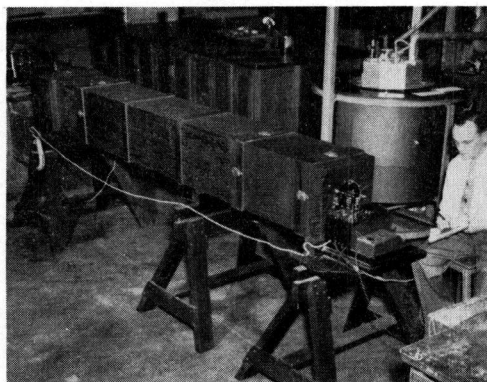
Figure 4. The Reflectometer Assembled for Measurements of Reflectance at 1 Deg. Divergence and 2 Deg. Incidence.
