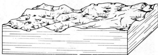
Figure 4. Limestone with sinkhole development. The roughly circular depressions result from the solution of limestone along cracks and fissures which are enlarged by percolating groundwater. They are often drained by subterranean streams but these are sometimes plugged and temporary ponds result. In tilted limestones, these depressions are interconnected and form long, shallow valleys along bedding planes.
