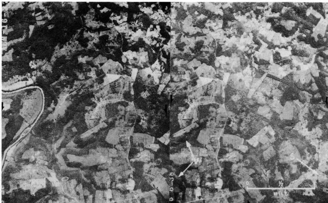
Figure 2. This view shows many features of a typical limestone area. In the upper portion a valley (without stream) has been formed by the complete collapse of a cavern system. It is worth spending extra time on this complex example to follow the process of analysis. The lower portion of the photo shows no sinks and a considerable amount of surface drainage. This indicates an impervious material (shale) rather than limestone at the surface. Since there is no sign of tilting of the rock, the deeply pitted valley at the top implies that the same limestone underlies the entire area. This is confirmed by: 1) steep-sided "limestone" valleys (V) cut through the shale and take on the features of the underlying rock; 2) sinks (beyond stereo-coverage) in fields at far right (S) and included in the bend of the river at left. The shale cap will eventually erode away and expose the limestone.
