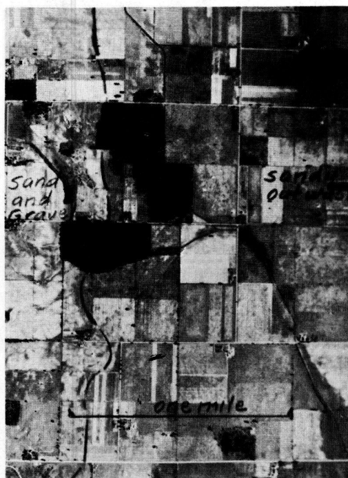
Figure 6. Airphoto of Sandy Outwash. The major portion of this photo is of the sandy outwash area in northwestern St. Joseph County in Indiana. It shows gently rolling to flat topography and light-gray color tones. Infiltration basins are faint and there are no gullies. The left portion of the picture bounded by the dashed line, shows the contrast of the more granular pattern. Figure 7 is illustrative of the topographic change at this boundary.
