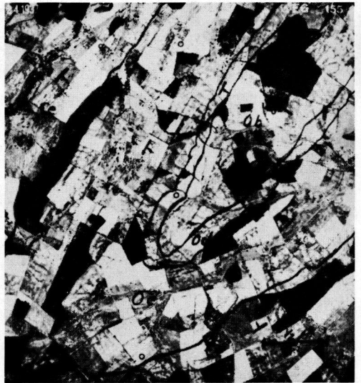
Figure 16. Airphoto showing syncline plunging southwestward. Notice convergence of sandstone ridges (wooded areas) within the Conococheague limestone. (Oc).
