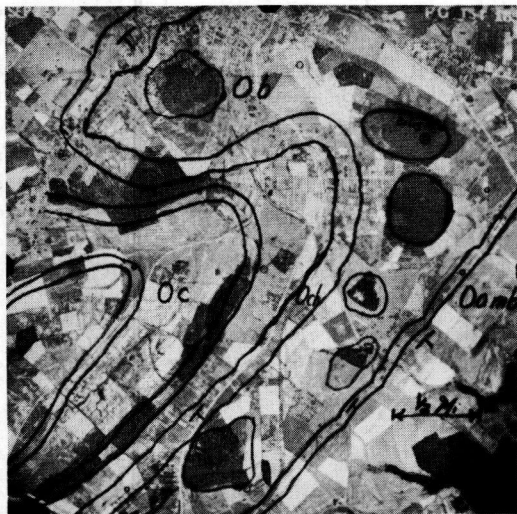
Figure 17. Airphoto showing features used in differentiating geologic formations in the area investigated. Notice cherty knolls (encircled areas) in Beekmantown formation (Ob) and the sandstone ridges (also encircled) in the Conococheague formation.
