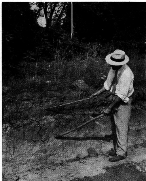
Figure 21. Profile of Iredell Soil. Large shrinkage cracks indicate expansive clay in the B-horizon (between pointers). Below is the sandy C-horizon.
