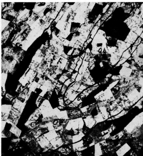
Figure 16. Airphoto showing syncline plunging southwestward. Notice convergence of sandstone ridges (wooded areas) within the Conococheague limestone. (Oc).
