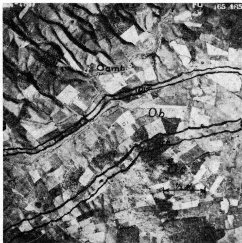
Figure 3. Airphoto showing contact of Athens and Martinsburg shale (Oamb) and Lenoir - Mosheim Limestone (Olm).
