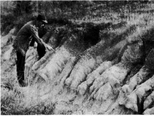
Figure 15. Erosion of typical Herndon soil profile. Dark color and shrinkage cracks indicate clay-like properties of B-horizon above the point indicated - C-horizon is below.
