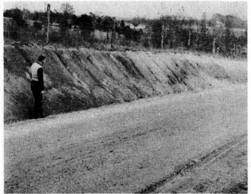
Figure 16. Deep uniform profile of Davidson Soil in foreground. Contrast at the second post indicates change to Herndon Soil.
