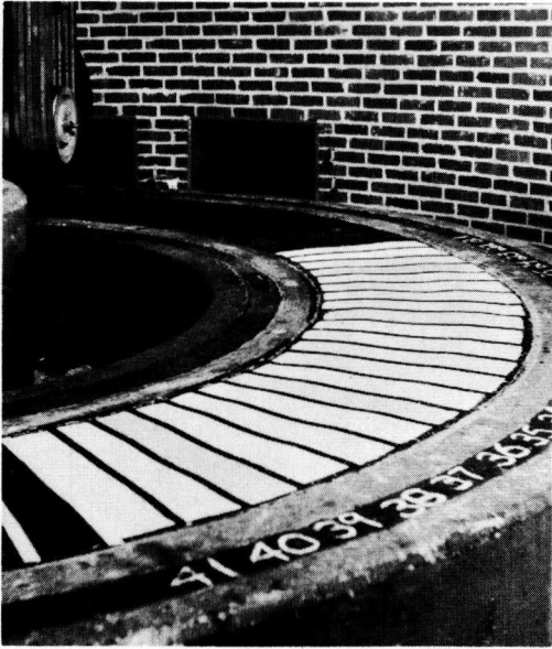
Figure 4. Accelerated-abrasion test. Paint segments are shown on the surface of the circular test tracks.
