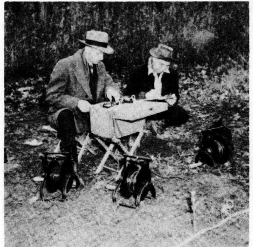
Figure 22. One type of resistivity apparatus using the Gish-Rooney commutator principle.
